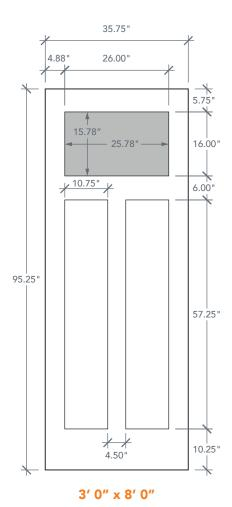
NOTE: BY REQUEST, DOOR HEIGHT COMES IN VARYING DIMENSIONS TO A MINIMUM OF 95". EXCESS WILL BE TAKEN FROM BOTTOM RAIL. ALL OTHER DIMENSIONS WILL REMAIN THE SAME.
